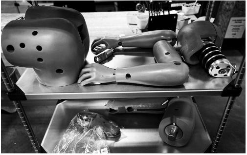
Hybrid III Dummy. Every part of a crash test dummy is designed to show how a real human body handles a crash.
